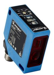
Wenglor photoelectric sensor, square, diffuse, Class 2 red laser, 30-80mm sensing distance, teach-in button, polycarbonate housing, 8-pin M12 quick-disconnect.
