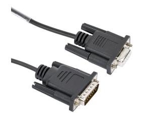
AutomationDirect communication cable, 15-pin D-shell male to 9-pin D-shell female, shielded, 2m/6.6ft cable length. For use with OP600 or OP1000 series Optimate units and a PC for programming or connecting to Allen-Bradley SLC5/03 and SLC5/04 CPUs.
