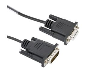
AutomationDirect communication cable, 15-pin D-shell male to 9-pin D-shell female, shielded, 2m/6.6ft cable length. For use with OP600 or OP1000 series Optimate units and a PC for programming or connecting to Allen-Bradley SLC5/03 and SLC5/04 CPUs.
