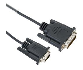
AutomationDirect communication cable, 15-pin D-shell male to 15-pin D-sub HD15 male, shielded, 2m/6.6ft cable length. For use with any OP600 or OP1000 series OptiMate unit and a DL06, or the bottom port of a D2-250(-1), D2-260 or D2-262 (bottom port) CPU.
