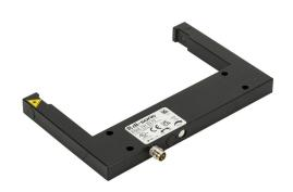
di-soric photoelectric fork sensor, U-frame, die-cast zinc housing, through-beam, Class 1 laser light emission, 0-120mm sensing distance, 10-30 VDC operating voltage, selectable light-on/dark-on, push-pull NPN or PNP, 3-wire, 3-pin M8 quick-disconnect.
