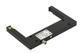
di-soric photoelectric fork sensor, U-frame, die-cast zinc housing, through-beam, Class 1 red laser, 0-120mm sensing distance, 10-30 VDC operating voltage, selectable light-on/dark-on, pushpull NPN or PNP, 3-wire, 3-pin M8 quick-disconnect.
