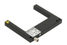
di-soric photoelectric fork sensor, U-frame, die-cast zinc housing, through-beam, Class 1 red laser, 0-80mm sensing distance, 10-30 VDC operating voltage, selectable light-on/dark-on, pushpull NPN or PNP, 3-wire, 3-pin M8 quick-disconnect.
