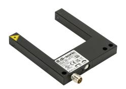
di-soric photoelectric fork sensor, U-frame, die-cast zinc housing, through-beam, Class 1 red laser, 0-50mm sensing distance, 10-30 VDC operating voltage, selectable light-on/dark-on, pushpull NPN or PNP, 3-wire, 3-pin M8 quick-disconnect.
