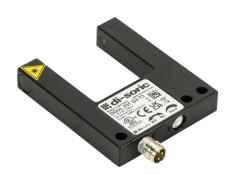
di-soric photoelectric fork sensor, U-frame, die-cast zinc housing, through-beam, Class 1 laser light emission, 0-30mm sensing distance, 10-30 VDC operating voltage, selectable light-on/dark-on, push-pull NPN or PNP, 3-wire, 3-pin M8 quick-disconnect.
