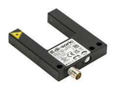
di-soric photoelectric fork sensor, U-frame, die-cast zinc housing, through-beam, Class 1 red laser, 0-30mm sensing distance, 10-30 VDC operating voltage, selectable light-on/dark-on, pushpull NPN or PNP, 3-wire, 3-pin M8 quick-disconnect.
