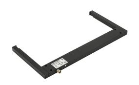
di-soric photoelectric fork sensor, U-frame, aluminum housing, through-beam, visible red, 0-250mm sensing distance, 10-30 VDC operating voltage, selectable light-on/dark-on, push-pull NPN or PNP, 3-wire, 3-pin M8 quick-disconnect.
