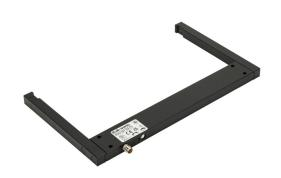
di-soric photoelectric fork sensor, U-frame, die-cast zinc housing, through-beam, visible red, 0-220mm sensing distance, 10-30 VDC operating voltage, selectable light-on/dark-on, push-pull NPN or PNP, 3-wire, 3-pin M8 quick-disconnect.
