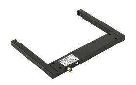
di-soric photoelectric fork sensor, U-frame, die-cast zinc housing, through-beam, visible red, 0-170mm sensing distance, 10-30 VDC operating voltage, selectable light-on/dark-on, push-pull NPN or PNP, 3-wire, 3-pin M8 quick-disconnect.
