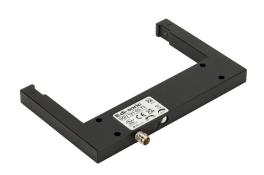
di-soric photoelectric fork sensor, U-frame, die-cast zinc housing, through-beam, visible red, 0-120mm sensing distance, 10-30 VDC operating voltage, selectable light-on/dark-on, push-pull NPN or PNP, 3-wire, 3-pin M8 quick-disconnect.
