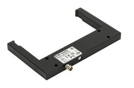
di-soric photoelectric fork sensor, U-frame, die-cast zinc housing, through-beam, infrared, 0-120mm sensing distance, 10-30 VDC operating voltage, selectable light-on/dark-on, push-pull NPN or PNP, 3-wire, 3-pin M8 quick-disconnect.
