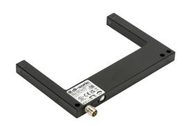
di-soric photoelectric fork sensor, U-frame, die-cast zinc housing, through-beam, visible red, 0-100mm sensing distance, 10-30 VDC operating voltage, selectable light-on/dark-on, push-pull NPN or PNP, 3-wire, 3-pin M8 quick-disconnect.
