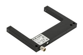
di-soric photoelectric fork sensor, U-frame, aluminum housing, through-beam, visible red, 0-90mm sensing distance, 10-30 VDC operating voltage, selectable light-on/dark-on, push-pull NPN or PNP, 3-wire, 3-pin M8 quick-disconnect.
