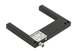
di-soric photoelectric fork sensor, U-frame, die-cast zinc housing, through-beam, visible red, 0-80mm sensing distance, 10-30 VDC operating voltage, selectable light-on/dark-on, push-pull NPN or PNP, 3-wire, 3-pin M8 quick-disconnect.
