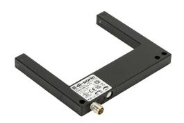
di-soric photoelectric fork sensor, U-frame, die-cast zinc housing, through-beam, infrared, 0-80mm sensing distance, 10-30 VDC operating voltage, selectable light-on/dark-on, push-pull NPN or PNP, 3-wire, 3-pin M8 quick-disconnect.
