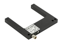
di-soric photoelectric fork sensor, U-frame, aluminum housing, through-beam, visible red light emission, 0-70mm sensing distance, 10-30 VDC operating voltage, selectable light-on/dark-on, push-pull NPN or PNP, 3-wire, 3-pin M8 quick-disconnect.
