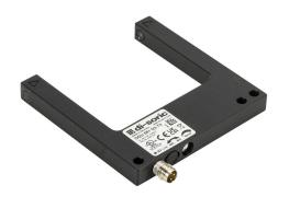
di-soric photoelectric fork sensor, U-frame, aluminum housing, through-beam, visible red, 0-60mm sensing distance, 10-30 VDC operating voltage, selectable light-on/dark-on, push-pull NPN or PNP, 3-wire, 3-pin M8 quick-disconnect.
