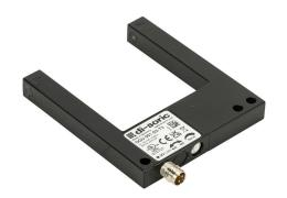
di-soric photoelectric fork sensor, U-frame, die-cast zinc housing, through-beam, visible red, 0-50mm sensing distance, 10-30 VDC operating voltage, selectable light-on/dark-on, push-pull NPN or PNP, 3-wire, 3-pin M8 quick-disconnect.
