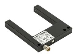
di-soric photoelectric fork sensor, U-frame, die-cast zinc housing, through-beam, infrared, 0-50mm sensing distance, 10-30 VDC operating voltage, selectable light-on/dark-on, push-pull NPN or PNP, 3-wire, 3-pin M8 quick-disconnect.
