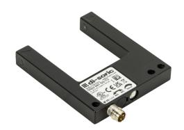
di-soric photoelectric fork sensor, U-frame, die-cast zinc housing, through-beam, visible red, 0-40mm sensing distance, 10-30 VDC operating voltage, selectable light-on/dark-on, push-pull NPN or PNP, 3-wire, 3-pin M8 quick-disconnect.
