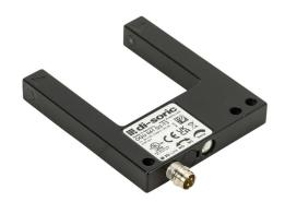
di-soric photoelectric fork sensor, U-frame, die-cast zinc housing, through-beam, visible red light emission, 0-40mm sensing distance, 10-30 VDC operating voltage, selectable light-on/dark-on, push-pull NPN or PNP, 3-wire, 3-pin M8 quick-disconnect.
