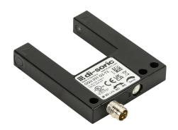
di-soric photoelectric fork sensor, U-frame, die-cast zinc housing, through-beam, visible red, 0-30mm sensing distance, 10-30 VDC operating voltage, selectable light-on/dark-on, push-pull NPN or PNP, 3-wire, 3-pin M8 quick-disconnect.
