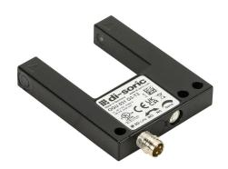
di-soric photoelectric fork sensor, U-frame, die-cast zinc housing, through-beam, visible red light emission, 0-30mm sensing distance, 10-30 VDC operating voltage, selectable light-on/dark-on, push-pull NPN or PNP, 3-wire, 3-pin M8 quick-disconnect.
