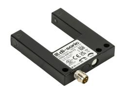
di-soric photoelectric fork sensor, U-frame, die-cast zinc housing, through-beam, infrared, 0-30mm sensing distance, 10-30 VDC operating voltage, selectable light-on/dark-on, push-pull NPN or PNP, 3-wire, 3-pin M8 quick-disconnect.
