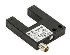
di-soric photoelectric fork sensor, U-frame, die-cast zinc housing, through-beam, visible red, 0-20mm sensing distance, 10-30 VDC operating voltage, selectable light-on/dark-on, push-pull NPN or PNP, 3-wire, 3-pin M8 quick-disconnect.
