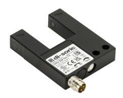
di-soric photoelectric fork sensor, U-frame, die-cast zinc housing, through-beam, infrared, 0-20mm sensing distance, 10-30 VDC operating voltage, selectable light-on/dark-on, push-pull NPN or PNP, 3-wire, 3-pin M8 quick-disconnect.
