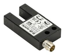
di-soric photoelectric fork sensor, U-frame, die-cast zinc housing, through-beam, infrared, 0-10mm sensing distance, 10-30 VDC operating voltage, selectable light-on/dark-on, push-pull NPN or PNP, 3-wire, 3-pin M8 quick-disconnect.
