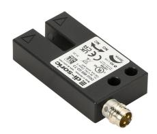
di-soric photoelectric fork sensor, U-frame, aluminum housing, through-beam, infrared, 0-5mm sensing distance, 10-30 VDC operating voltage, selectable light-on/dark-on, push-pull NPN or PNP, 3-wire, 3-pin M8 quick-disconnect.
