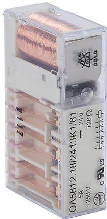
Dold force guided relay, socket mount, encapsulated, 24 VDC coil voltage, 6PST, (3) N.O., (3) N.C., 5A contact rating, 14-pin. Requires HL3096N-102-24 mounting socket.
