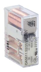
Dold force guided relay, socket mount, encapsulated, 24 VDC coil voltage, 4PST, (2) N.O., (2) N.C., 5A contact rating, 10-pin. Requires HC3096N-102-24 mounting socket.
