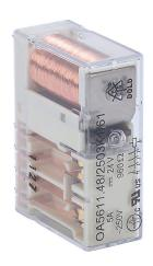
Dold force guided relay, socket mount, encapsulated, 24 VDC coil voltage, 4PST, (3) N.O., (1) N.C., 5A contact rating, 10-pin. Requires HC3096N-102-24 mounting socket.
