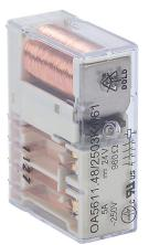
Dold force guided relay, socket mount, encapsulated, 24 VDC coil voltage, 4PST, (3) N.O., (1) N.C., 5A contact rating, 10-pin. Requires HC3096N-102-24 mounting socket.
