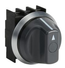
Schmersal selector switch, IP67 and IP69K, 22mm, 3-position, spring return to center from right, maintained left, operator only, plastic base, plastic bezel, Operator: black, knob, 44mm, round, plastic. Requires contact blocks.
