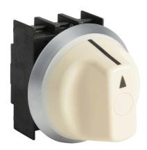
Schmersal selector switch, IP67 and IP69K, 22mm, 3-position, spring return to center from right, maintained left, operator only, plastic base, plastic bezel, Operator: white, knob, 44mm, round, plastic. Requires contact blocks.
