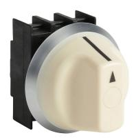
Schmersal selector switch, IP67 and IP69K, 22mm, 3-position, spring return to center from left, maintained right, operator only, plastic base, plastic bezel, Operator: white, knob, 44mm, round, plastic. Requires contact blocks.
