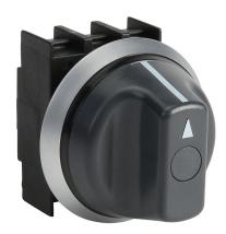
Schmersal selector switch, IP67 and IP69K, 22mm, 3-position, spring return to center from right or left, operator only, plastic base, plastic bezel, Operator: black, knob, 44mm, round, plastic. Requires contact blocks.
