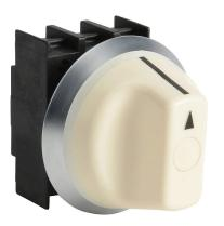
Schmersal selector switch, IP67 and IP69K, 22mm, 3-position, spring return to center from right or left, operator only, plastic base, plastic bezel, Operator: white, knob, 44mm, round, plastic. Requires contact blocks.
