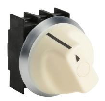
Schmersal selector switch, IP67 and IP69K, 22mm, 2-position, spring return from right, operator only, plastic base, plastic bezel, Operator: white, knob, 44mm, round, plastic. Requires contact blocks.
