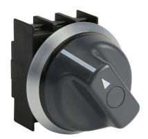
Schmersal selector switch, IP67 and IP69K, 22mm, 2-position, maintained, operator only, plastic base, plastic bezel, Operator: black, knob, 44mm, round, plastic. Requires contact blocks.
