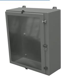
Stahlin N series enclosure, NEMA 1/3/3R/4X/12, 36 x 30 x 12in (HxWxD), wall mount, fiberglass reinforced polyester, gray, single-door, (5) twist-lock latches, padlock hasp and staple, SAR acrylic window.
