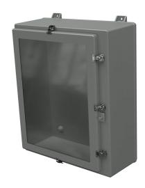
Stahlin N series enclosure, NEMA 1/3/3R/4X/12, 30 x 24 x 10in (HxWxD), wall mount, fiberglass reinforced polyester, gray, single-door, (5) twist-lock latches, padlock hasp and staple, SAR acrylic window.
