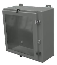
Stahlin N series enclosure, NEMA 1/3/3R/4X/12, 24 x 24 x 10in (HxWxD), wall mount, fiberglass reinforced polyester, gray, single-door, (4) twist-lock latches, padlock hasp and staple, SAR acrylic window.
