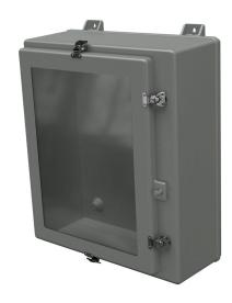
Stahlin N series enclosure, NEMA 1/3/3R/4X/12, 24 x 20 x 8in (HxWxD), wall mount, fiberglass reinforced polyester, gray, single-door, (4) twist-lock latches, padlock hasp and staple, SAR acrylic window.
