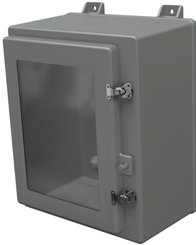
Stahlin N series enclosure, NEMA 1/3/3R/4X/12, 20 x 16 x 10in (HxWxD), wall mount, fiberglass reinforced polyester, gray, single-door, (2) twist-lock latches, padlock hasp and staple, SAR acrylic window.
