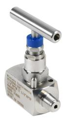
Winters manual isolation and throttling needle valve, straight body hard seat, single handle, stainless steel body, 1/4in male NPT inlet(s), 1/4in female NPT outlet(s).
