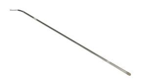
ProSense temperature sensor, 10K Type 3 thermistor, lead wire transition probe, 18in insertion length, 1/4in probe diameter, stainless steel sheath, 6ft 24 AWG wire leads.
