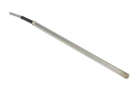
ProSense temperature sensor, 10K Type 3 thermistor, lead wire transition probe, 6in insertion length, 1/4in probe diameter, stainless steel sheath, 6ft 24 AWG wire leads.
