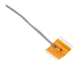
ProSense temperature sensor, 10K Type 3 thermistor, spade sensor, flexible polyimide with adhesive tape backing, 6ft 24 AWG wire leads.
