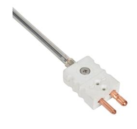
ProSense temperature sensor, 10K Type 3 thermistor, attached plug probe, 18in insertion length, 1/4in probe diameter, stainless steel sheath, 2-pin standard size plug.
