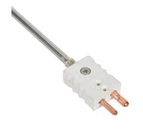
ProSense temperature sensor, 10K Type 3 thermistor, attached plug probe, 12in insertion length, 1/4in probe diameter, stainless steel sheath, 2-pin standard size plug.
