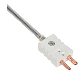
ProSense temperature sensor, 10K Type 3 thermistor, attached plug probe, 6in insertion length, 1/4in probe diameter, stainless steel sheath, 2-pin standard size plug.
