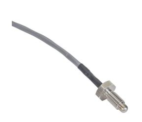
ProSense temperature sensor, 10K Type 3 thermistor, threaded bolt sensor, 3/8in bolt length, 3/16in tip, stainless steel sheath, 1/4-28 UNF process connection, 6ft 24 AWG wire leads.
